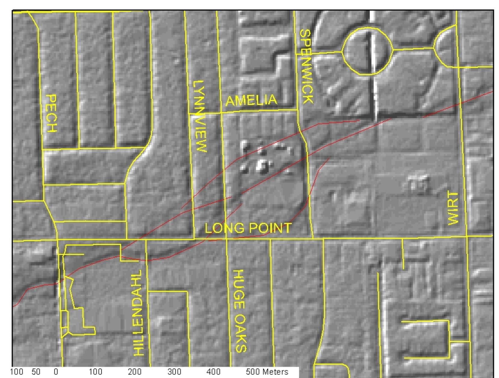
LIDAR hillshade image of Long Point fault where it crosses Long Point. Here the scarp splits into several branches.
